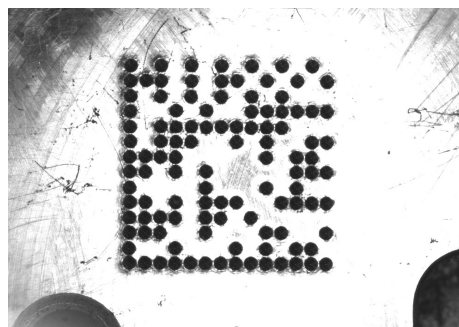
Figure 4-3 GS1 DataMatrix dot-peen symbol
